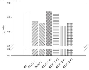
**Figure 5.** Ratio of cellulose Iα in various BC polysaccharide mats as determined by FTIR spectroscopy according to the methods of Tokoh. [6,7]
