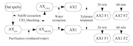
**Figure 1.**Diagram of the extraction and fractionation steps of the oat spelt arabinoxylan also illustrating the abbreviations used for the different arabinoxylan fractions.
