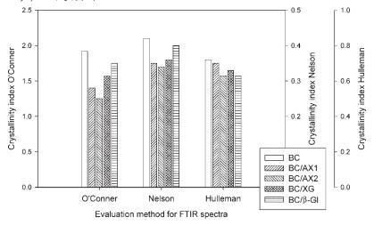
**Figure 4.** Crystallinity index of cellulose from various BC/polysaccharide mats as determined by FTIR spectroscopy according to the methods of O'Conner ( $A_{1429}/A_{897}$ ), Nelson ( $A_{1372}/A_{2900}$ ), and Hulleman ( $A_{1280}/A_{1200}$ ). [26-28] (see Figure 1 for abbreviations).
